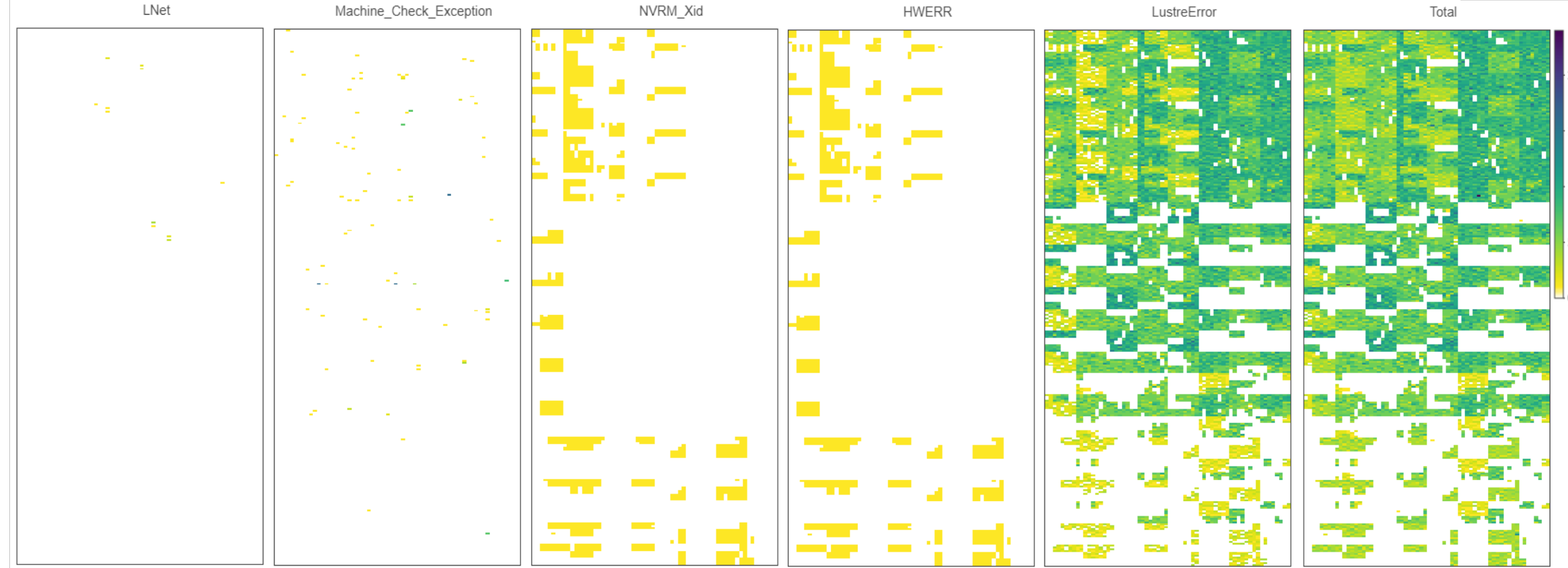
Figure 3: The nodal layouts for every event type and the combined total for one-hour window prior to "2015-02-09 01:49:54". Each layout has dimensions of [300, 64] in pixel and each pixel represents a unique Titan node with its coordinates [X, Y] (definition in following section).
